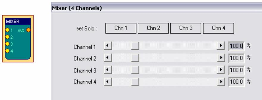
The *Mixer* - element can be used to merge up to four input signals into one output signal. The amplification-ratios are given with the corresponding sliders. Using the buttons Chn1 - Chn4, presets for solo-output of the selected channel are activated.
