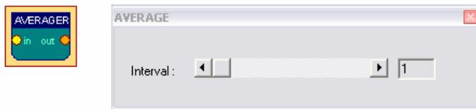
The *Averager* element puts out the mathematical average of the last  $n$  samples. The number of samples can be selected by the Interval scroll bar. If 0 is selected, all samples will be averaged (this can be useful to accumulate data for a whole session).
