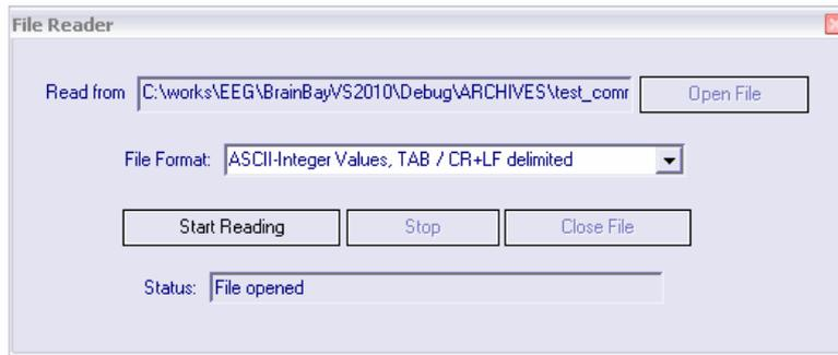
The *File-Reader* element can be used to read channel data from a text file. Using the *File Format* combo box, the type of storage and the delimiters for rows and columns can be selected. For more information please see the File Writer description.
