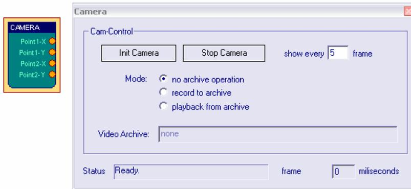
To use the camera element, a webcam or another camera needs to be connected and visible to the system (installation of correct device drivers etc). After inserting the camera element into the design, the device is opened and the live-stream is displayed in a separate window.
