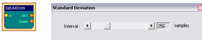
This Element calculates standard deviation and mean of  $n$  samples and puts the results to the output ports. The number of samples for the calculation interval can be set using the slider bar.
