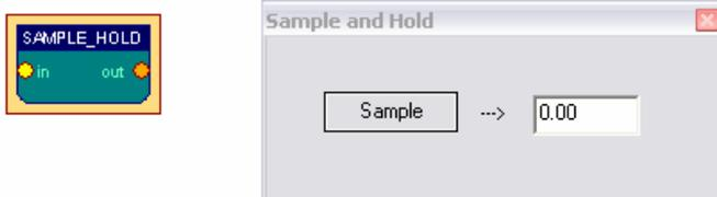
The *Sample-Hold* - element stores the current input-value when the button *Sample* is pressed. This value will be present at the output-port until another value is stored using the button.
