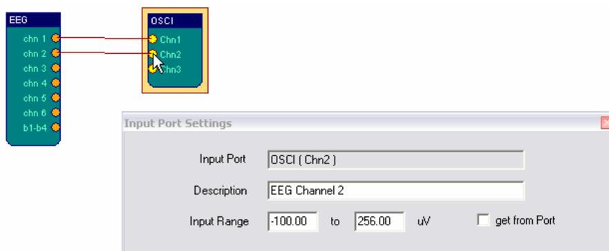
The *Input-Port Dialog* for the oscilloscope-element (channel 2). The input-range for the specific port can be adjusted or inherited from the connection. Adjusting the input-range would make sense when a smaller range has to be displayed etc.
